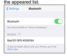
Select the external device and pair it with your mobile device. To do so, select *Pair* on your device and on Bad Elf receiver.
